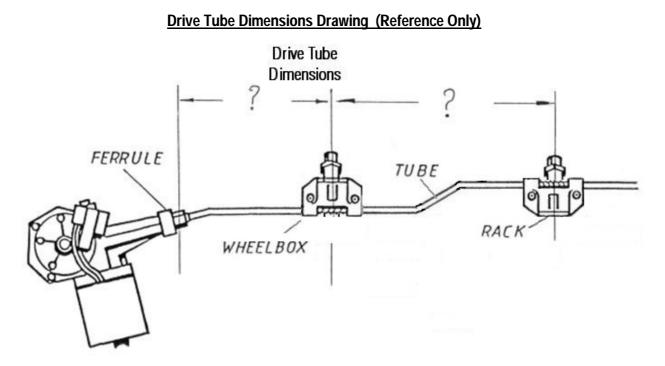
Note for centre parking blades, i.e. like FX/FJ Holden's, the LHS wheelbox is reversed and its drive cable and Tube runs under the bottom of the wheelbox and the centre tube is bent in a slight s bend to bring it back up to the top the RH Wheelbox.
