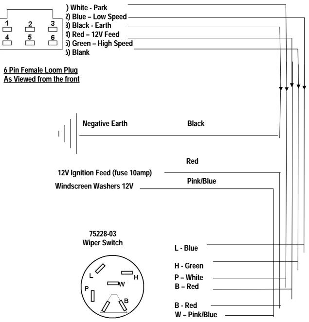
Wiper switch system is 12V Positive Feed
