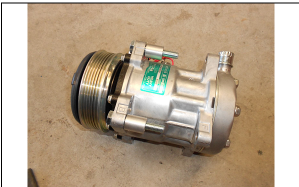
Picture 6 - Notice the position of the bushes for installing compressor unit to an LS1 or 2
