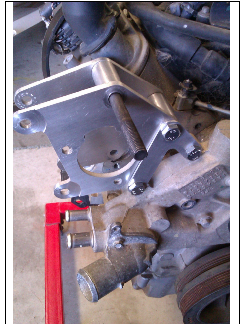
Picture 3 - Mounting A/C bracket assembly to the head and water pump
