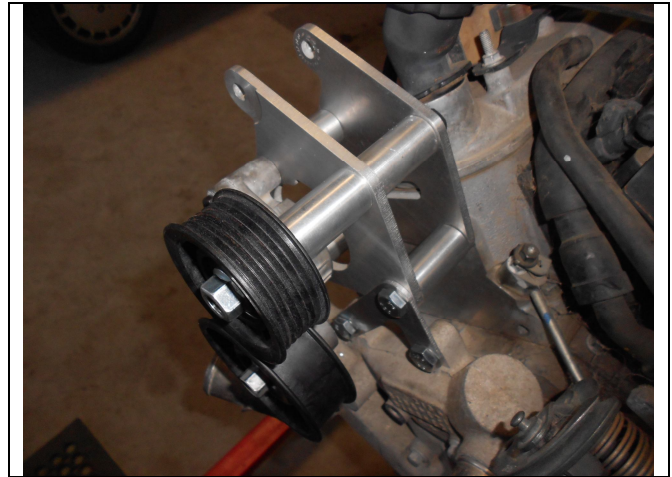
Picture 5 – The Idler and tensioner located on the mounting bracket assembly
